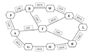
STEP 1: Mark the source node with a current distance of 0 and the rest with infinity.
